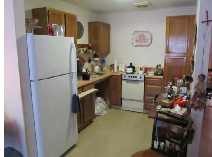
Handicap accessible unit kitchens include required knee clearance space under the sink
